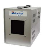
The BL671 is a small size blackbody calibration source utilizing a digital indicating temperature ambient 30°C to 50°C (86F to 122F). A 70x70 mm size ridged plate is heated or cooled with an internal solid state thermoelectric heat pump. It has a built-in digital temperature controller to provide accurate, stable temperature as well as to provide readout.
